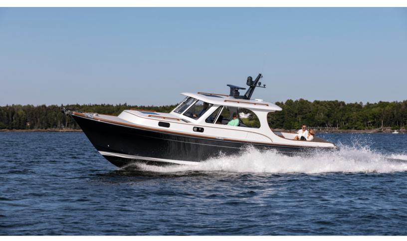
Shadow, the first vessel in the new Hood 35 LM series, features twin YANMAR 6LY440s coupled to a pair of Hamilton Waterjet HJX29s. Credit: Lyman-Morse
