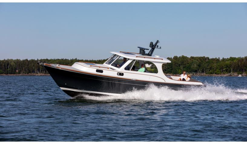
Shadow, the first vessel in the new Hood 35 LM series, features twin YANMAR 6LY440s coupled to a pair of Hamilton Waterjet HJX29s. Credit: Lyman-Morse
