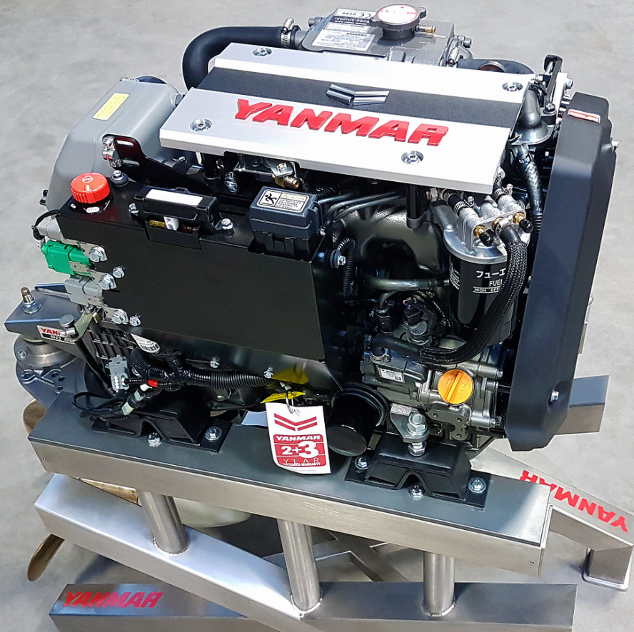
The YANMAR 3JH40 engine - the world's smallest common rail inboard marine diesel engine
