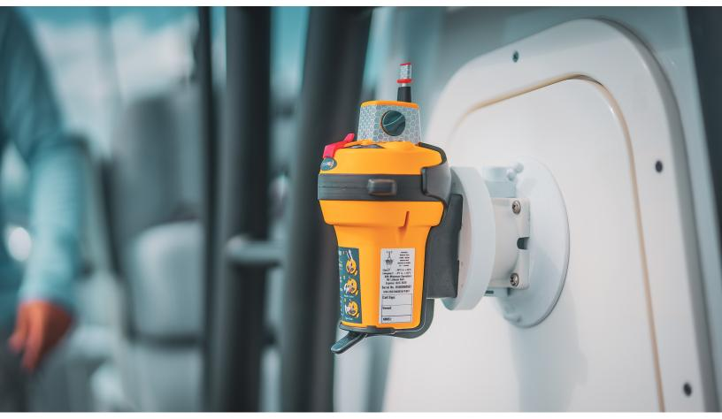
EPIRBs, such as the Ocean Signal rescueME EPIRB1, are installed on the boat to alert search and rescue in an emergency
