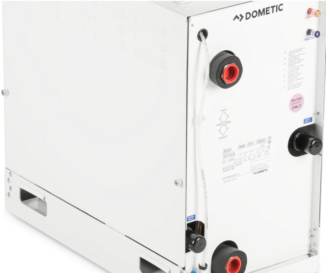
Dometic VARCX60 variable capacity chiller with titanium condenser coils
