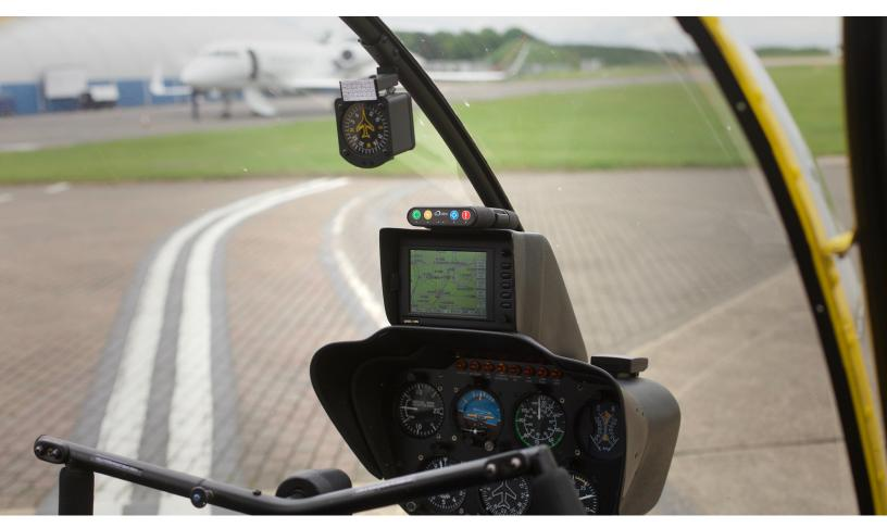
RockAIR is a dashboard mounted tracking, communication and IoT solution providing dual mode operation over satellite and GSM
