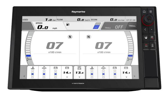
Raymarine's Axiom MFD series can now display the instrumentation for up to 4 Yamaha outboard engines on a single display.
