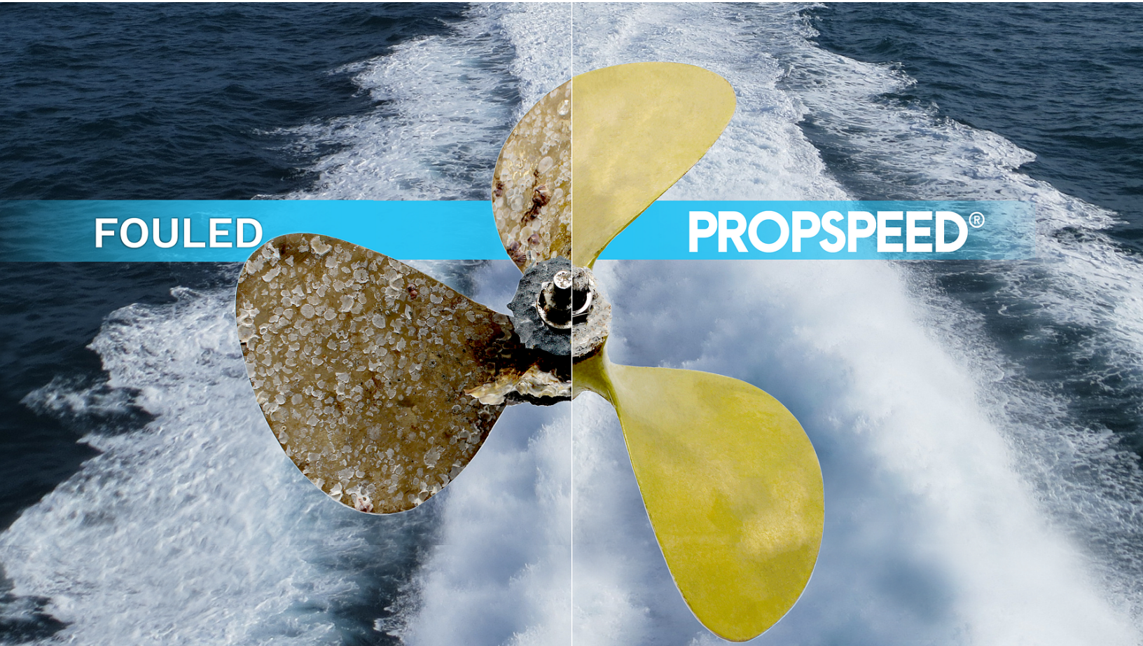
Propellers half coated with Prospeed and half without coating
