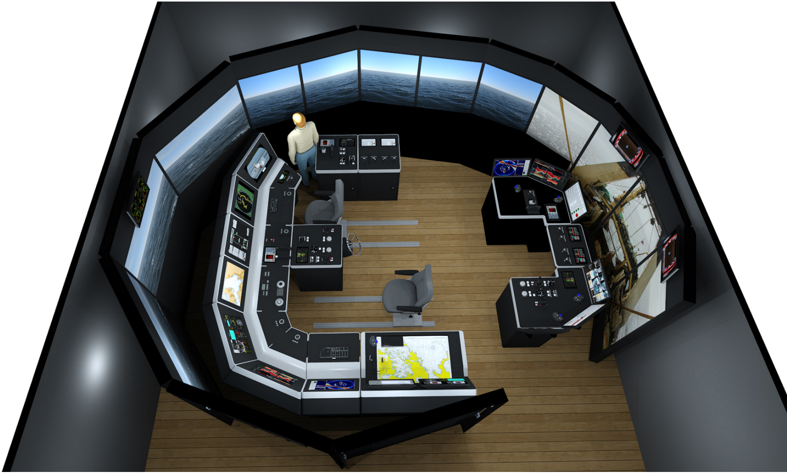
Illustration of a full mission K-Sim Fishery simulator with new purse seine functionality for studies and training
