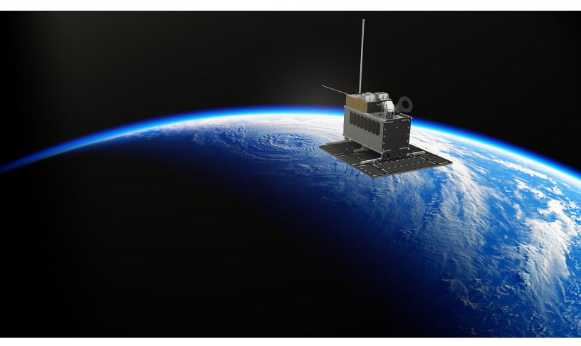
NorSat-3 carries AIS and radar detection payloads developed by or in collaboration with KONGSBERG
