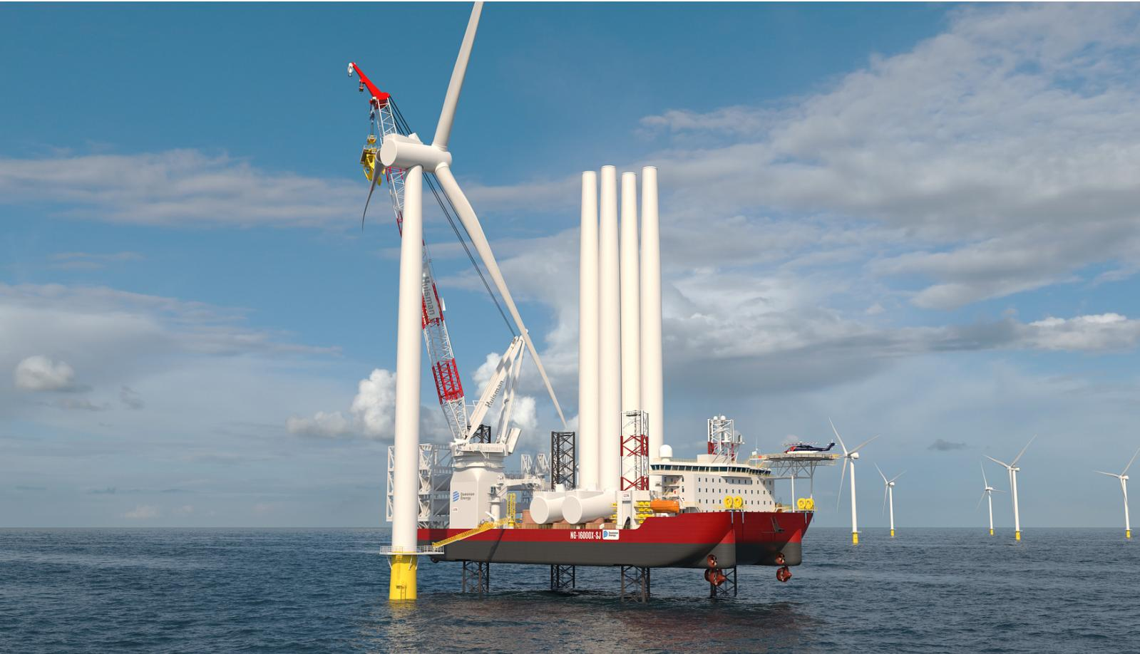
Dominion Energy's new Wind Turbine Installation Vessel, due for delivery by the end of 2023, will be built by Keppel AmFELS and fitted with Kongsberg Maritime's field-proven integrated solution for WTIV operation
