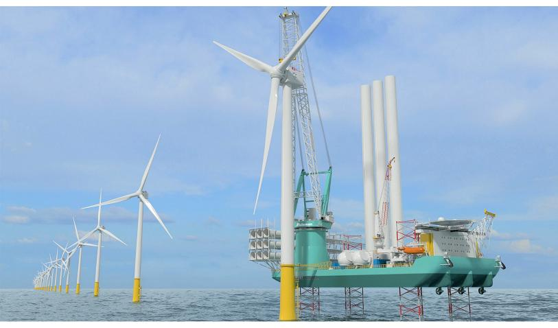
Equipped with Kongsberg Maritime systems, OIM Wind's new vessel will, on completion, be capable of sustainably transporting and installing multiple sets of next-generation wind turbines
