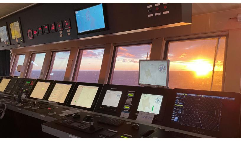
The KONGSBERG Integrated control system keeps the vessel's position, monitors and controls vessel functions and actively distributes energy across onboard consumers
