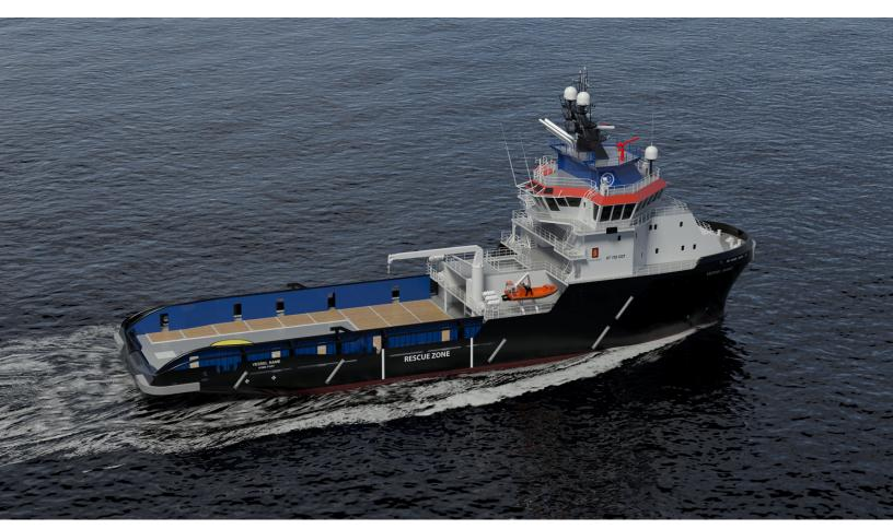
Kongsberg Maritime's 71.6-metre UT 722 tugboat design has bollard pull of 200 tonnes and can operate as a long-range towing vessel in the Suez Canal and the Mediterranean Sea
