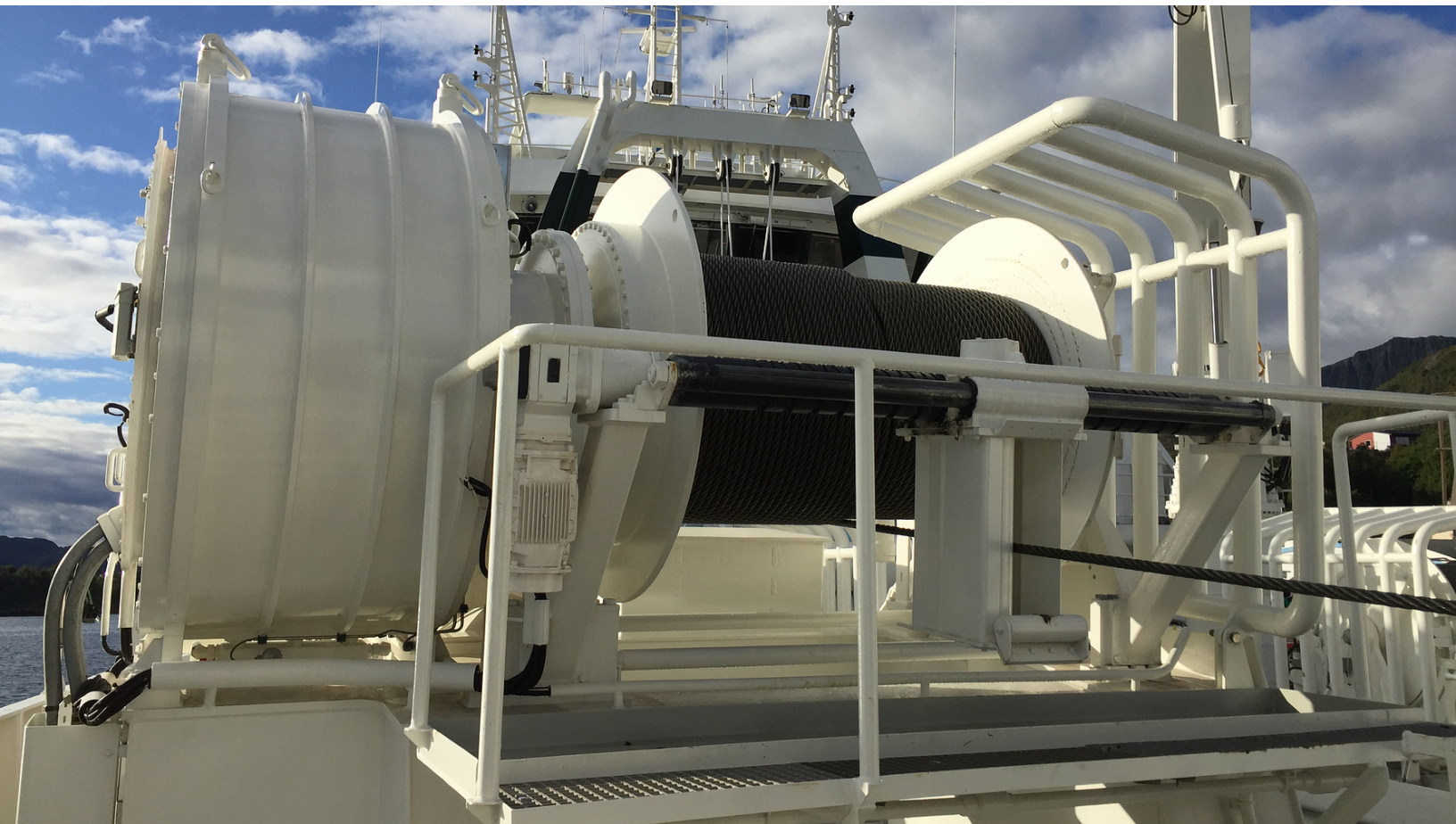
Kongsberg Maritime's EasyDrive electric trawl winch, installed on board the stern trawler Granit
