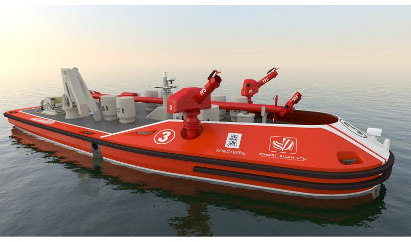
The first in the series will be the 20 m RALamander 2000, equipped with Fi Fi 1 capability, with a total pumping capacity of 2400 m3/hr with optional foam
