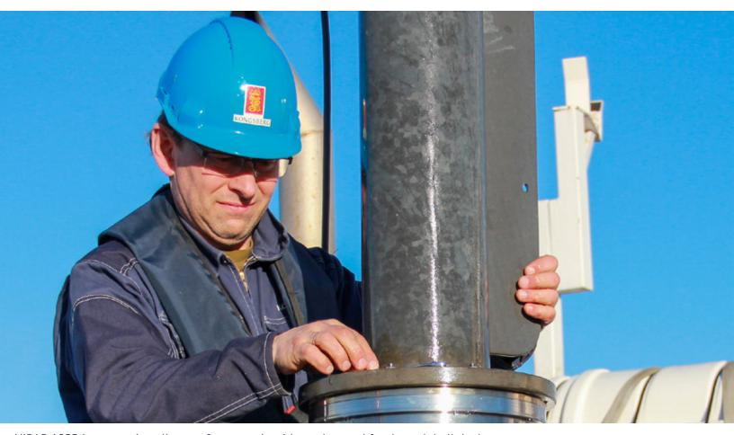
HiPAP 102P is easy to install on surface vessels without the need for through hull deployment
