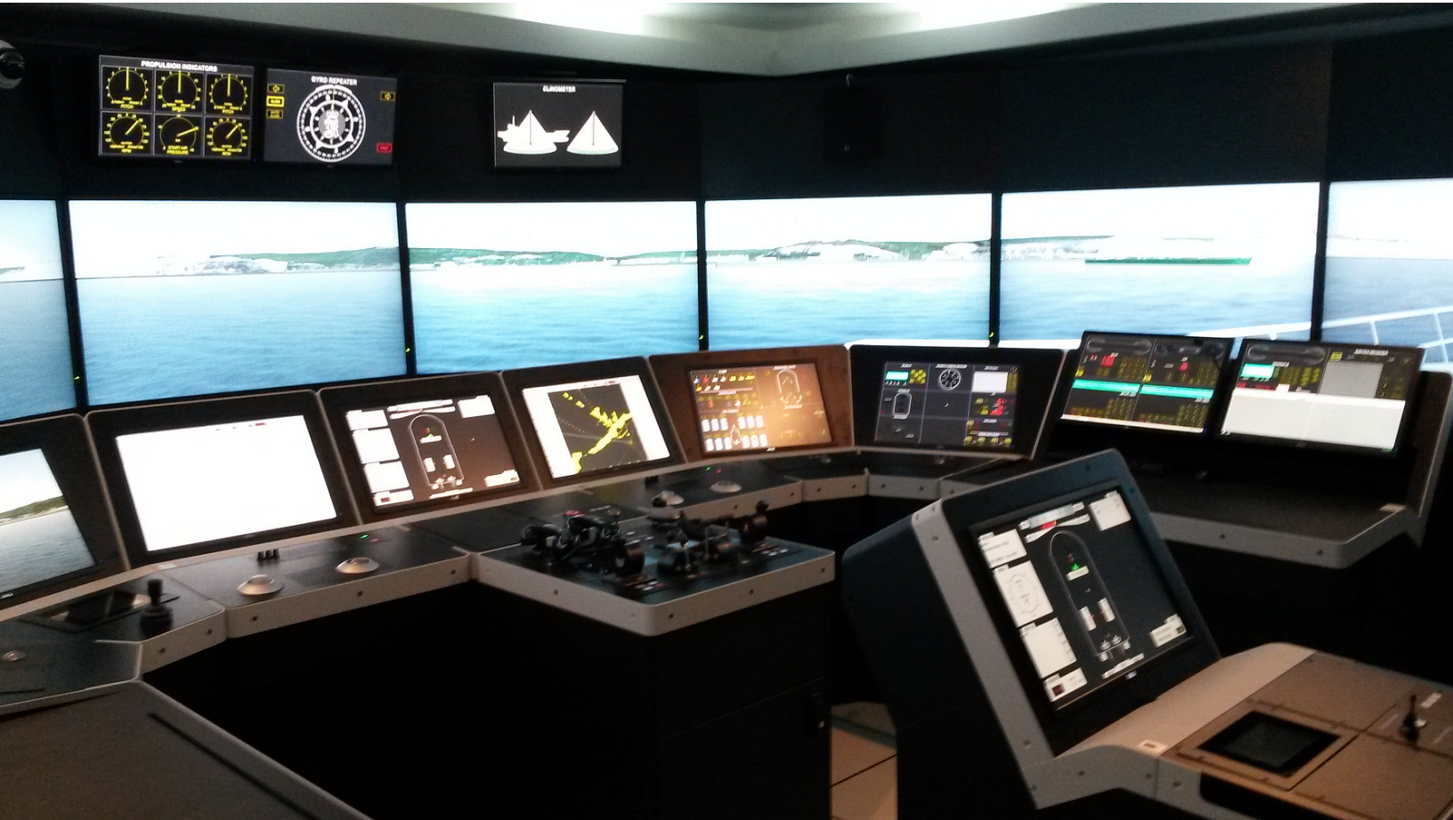
New KONGSBERG simulator at the Ministry of Transportation's Maritime Training Centre in Jakarta
