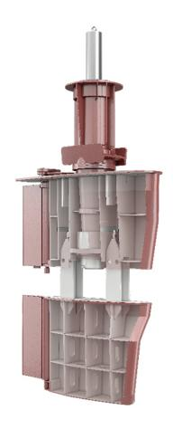
Kongsberg Maritime's new Direct Trunk Support rudder system reduces the forces from manoeuvring to the steering system
