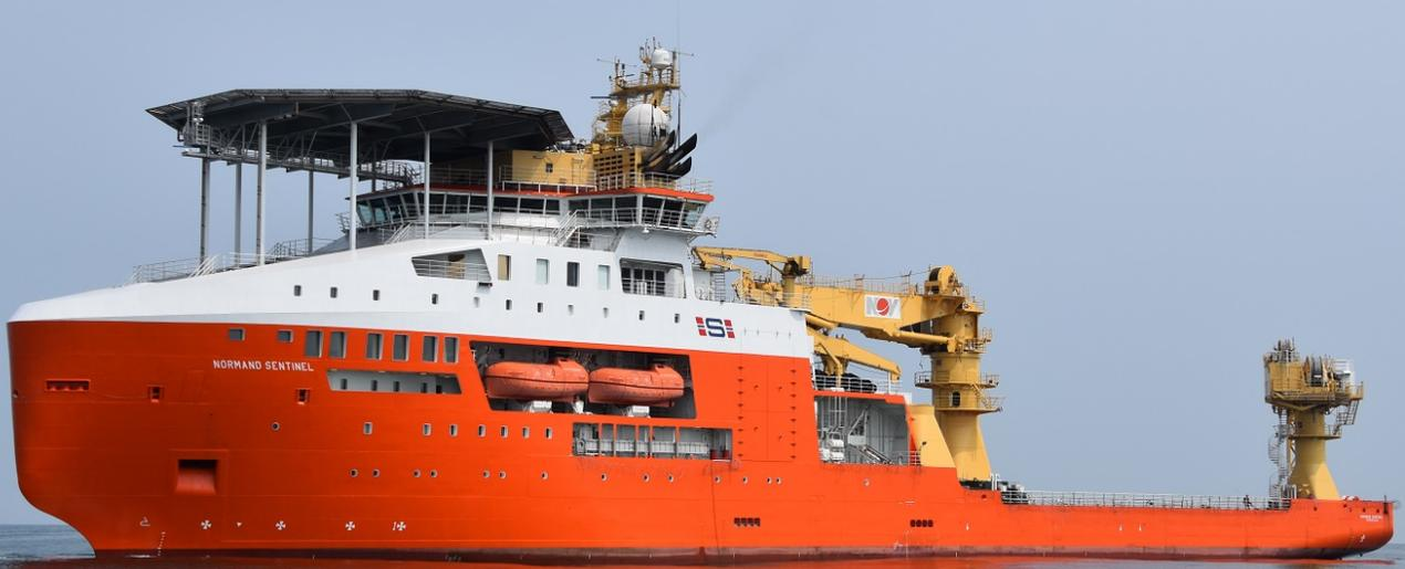
Solstad's Normand Sentinel will transition to Kongsberg Maritime's state-of-the-art electric rim-drive azimuth thrusters as part of a significant upgrade to increase energy efficiency
