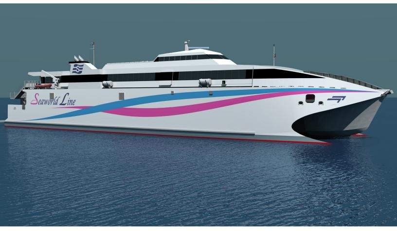
Incat's new wave piercing 'Hull 097' will be powered by four Kongsberg Kamewa S90-4 waterjets
