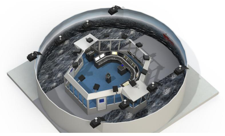
Illustration of K-Sim Navigation DNV GL Class A bridge simulator with 360 degrees field of view, scheduled for delivery to Simwave's brand new training facility in Barendrecht, The Netherlands at the end of September 2017
