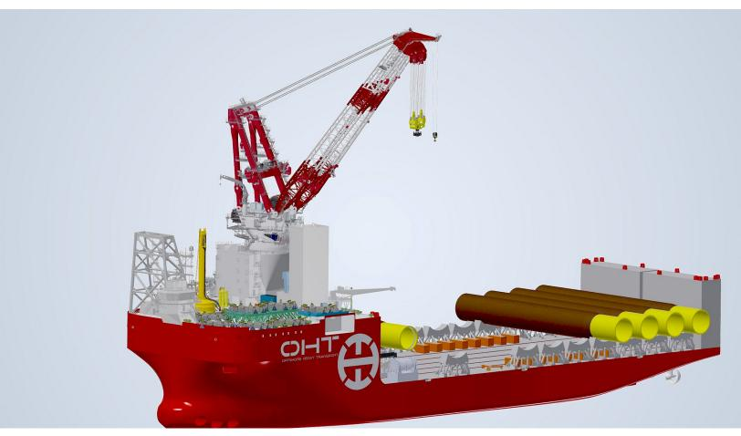
Kongsberg Maritime is to supply a PGGS for the Ulstein-designed OHT Alfa Lift offshore wind foundation installation vessel
