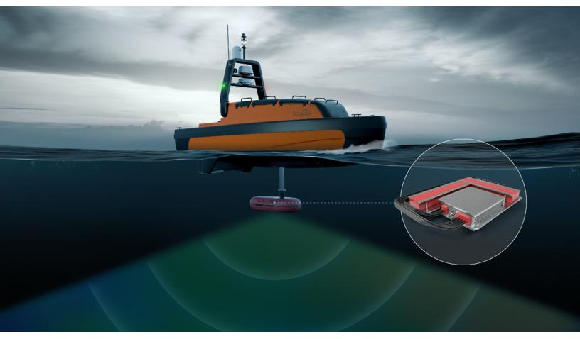
Kongsberg Maritime's latest addition to the EM 712 range of multibeam echosounders is an ideal solution for USVs as its swath coverage is fully stabilised for roll, pitch and yaw
