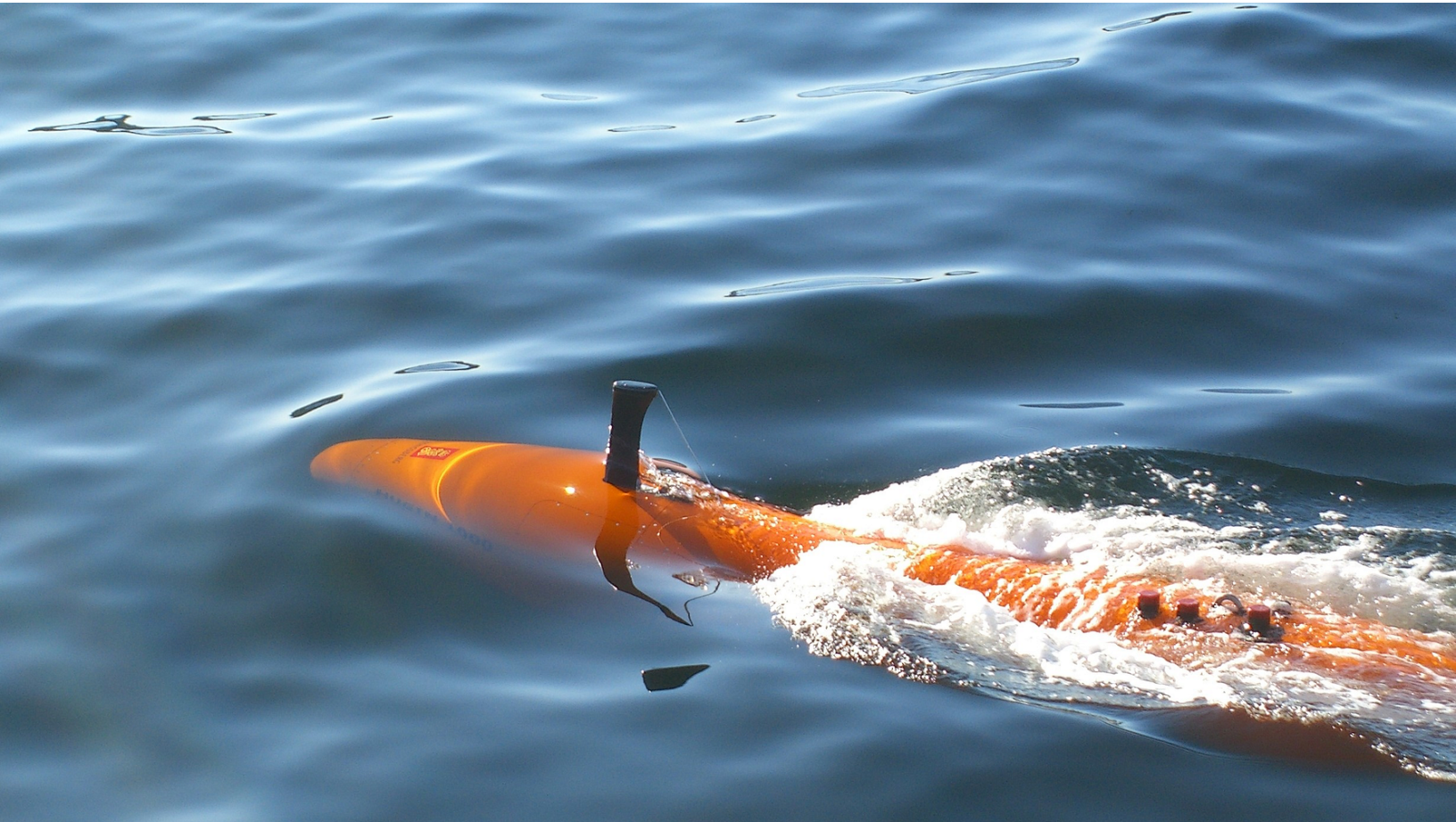
A Kongsberg Maritime HUGIN Autonomous Underwater Vehicle (AUV) at the surface
