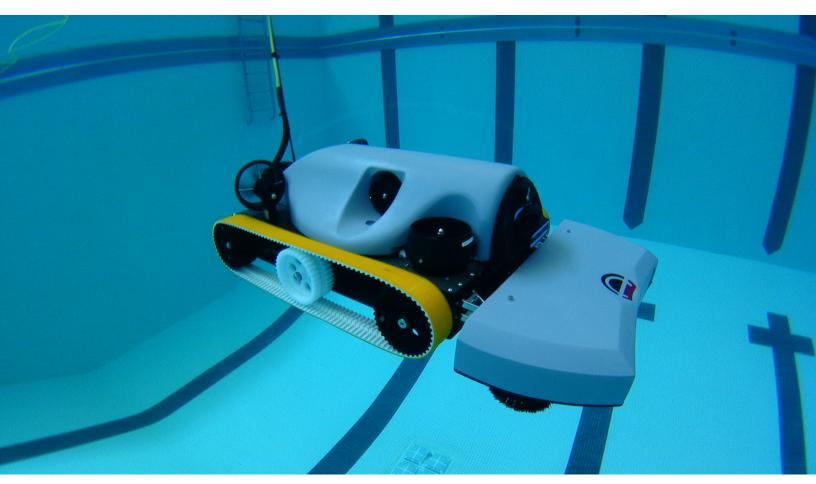
Proactive in-water hull cleaning capability
