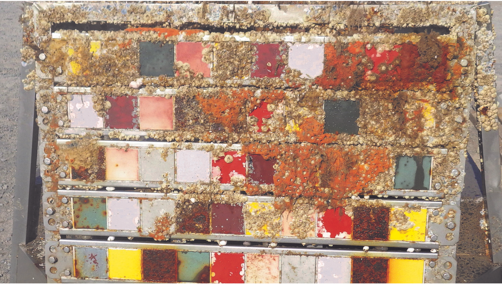
Coppercoat (green) showed minimal fouling and erosion after five years
