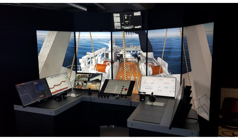
The new K-Sim Fishery simulator includes instruments and aft deck view enabling training to avoid risk elements associated with aft deck operations onboard fishing vessels
