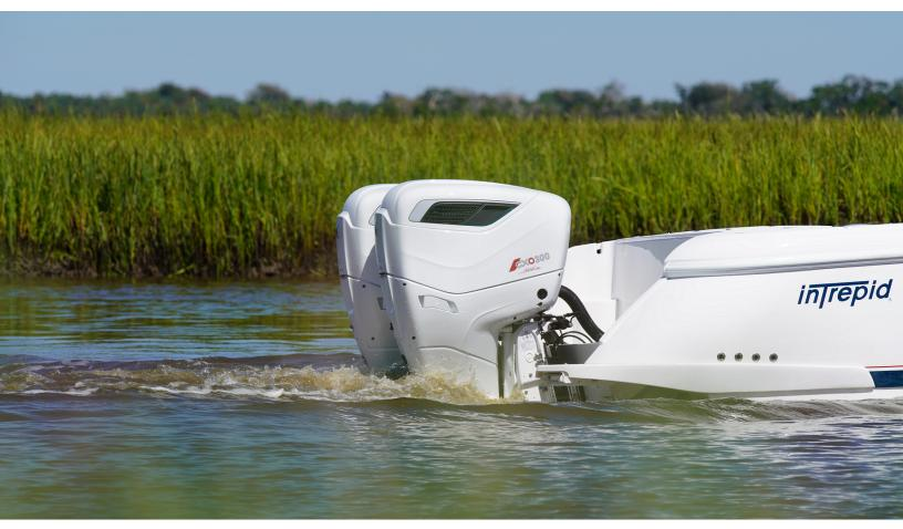
Cox Marine has brought the production of the PTT (power, tilt and trim) in-house to maintain the highest standards and keep up with demand for the CXO300 diesel outboard engine
