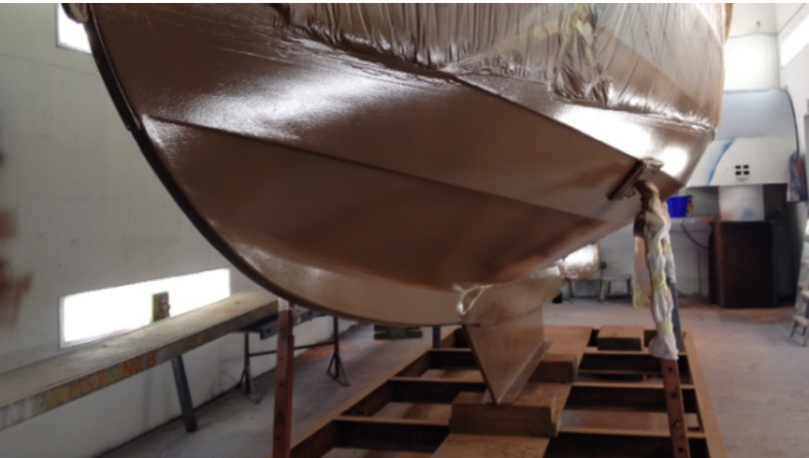
Coppercoat - application process
