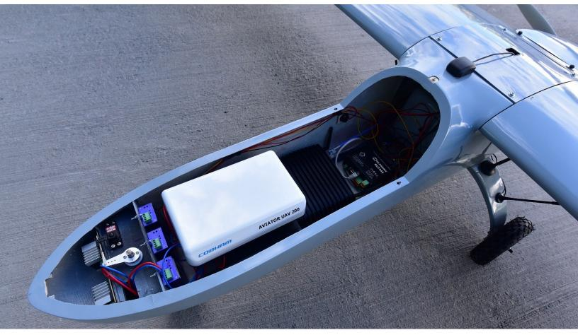
Cobham SATCOM's AVIATOR UAV 200 is the world's smallest and lightest Inmarsat UAV satcom solution, pictured installed in AnsuR-Nexus
