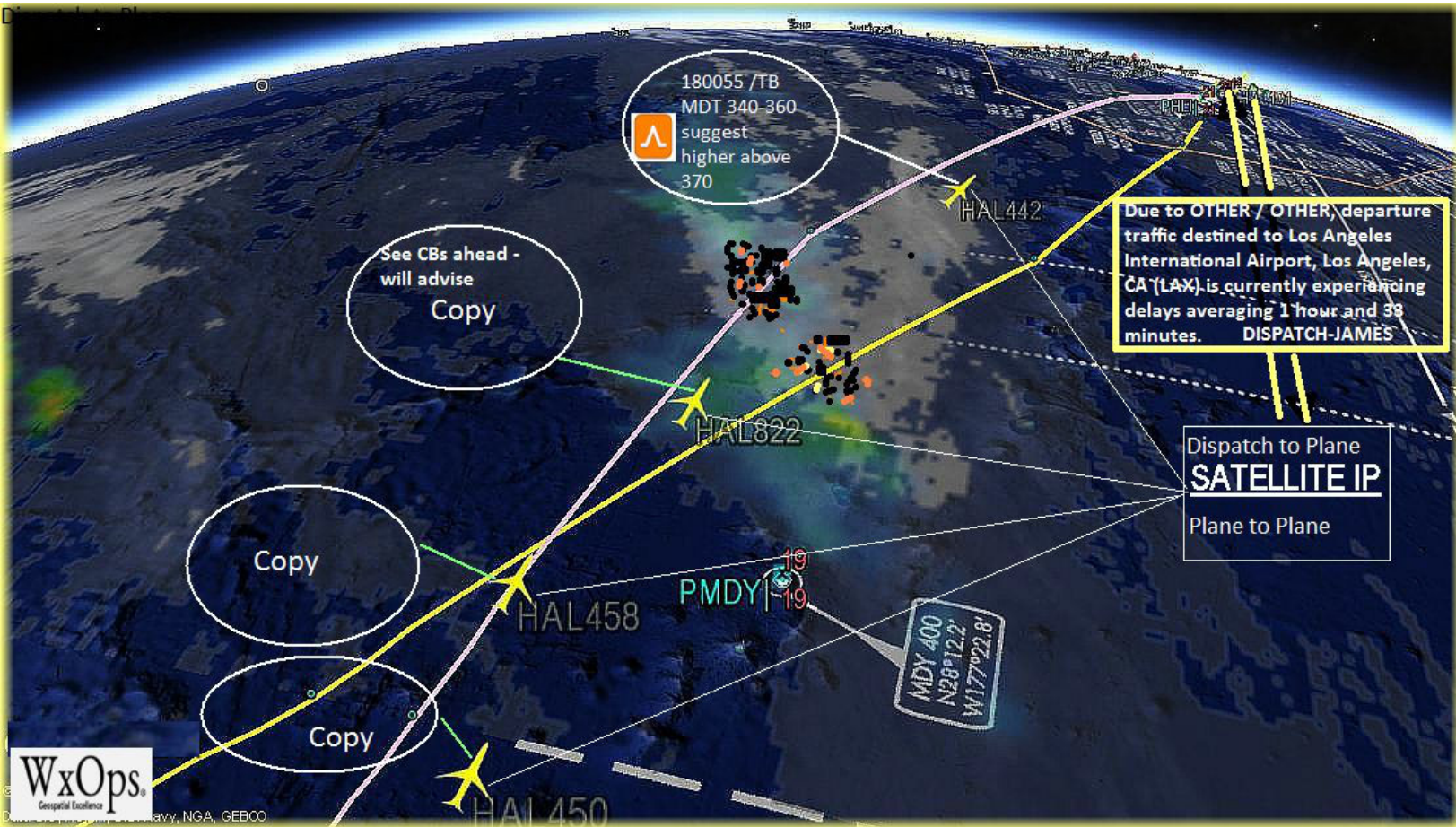
WxOps satellite enabled dispatcher & plane to plane communications network
