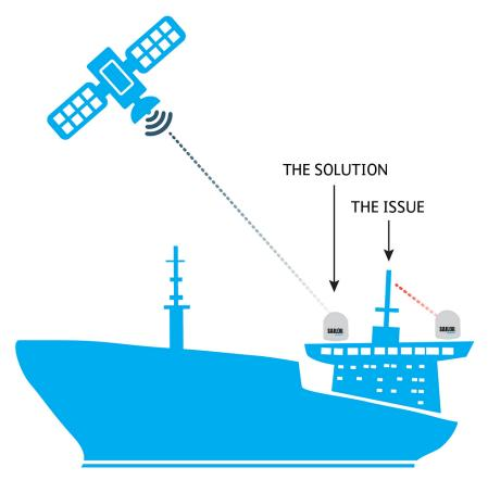
The new GX Antenna Diversity Solution overcomes link losses caused by satellite blocking from the ship structure or other deck equipment.
