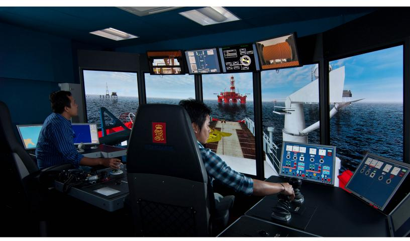
K-Sim Offshore with integrated Kongsberg Dynamic Positioning system is specially designed for advanced offshore operations and will be vital in JMI's future training programs.
