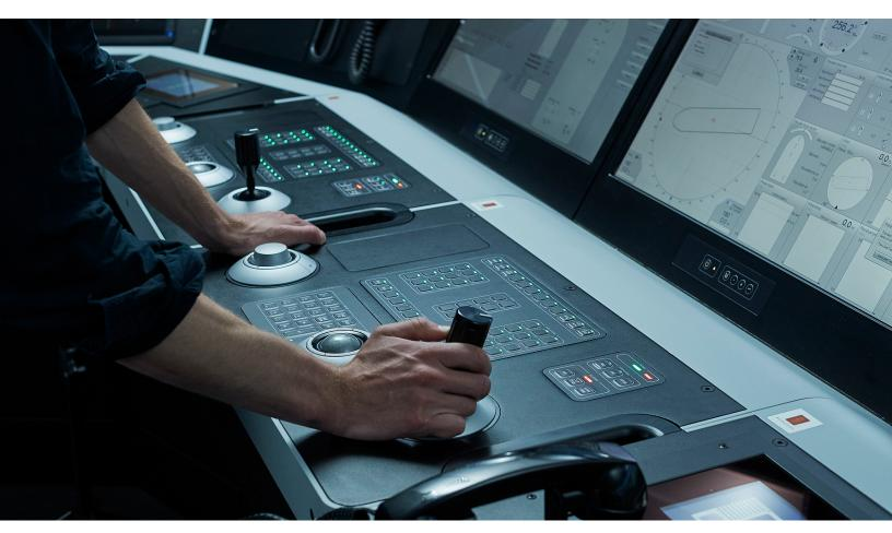
K-Sim DP Maneuvering simulators, as will be delivered to CERONAV, comprise a dual redundant K-Pos DP operator station, a DP controller and an independent joystick system
