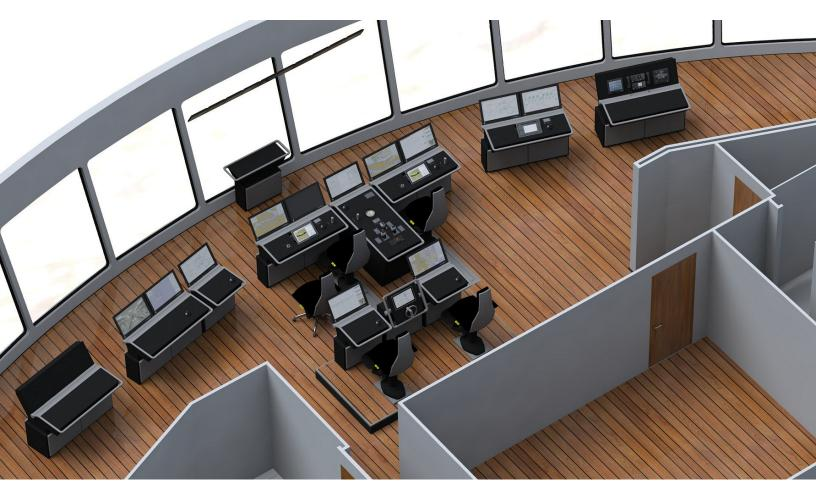
K-Bridge Integrated Bridge System (IBS) with K-Pos Dynamic Positioning (DP) functionality for two ultra-luxury, purpose-built expedition cruise newbuilds
