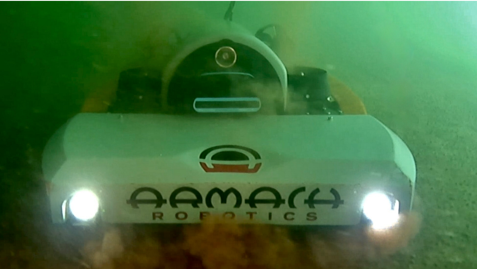
Armach Robotics HSR (Hull Service Robot) on a ship's hull.
