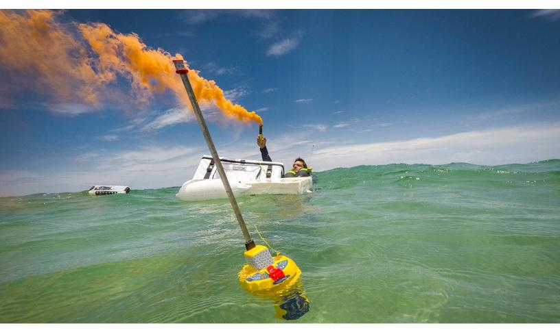
406 MHz beacons, such as the Ocean Signal EPIRB, provide access to rescue services in an emergency
