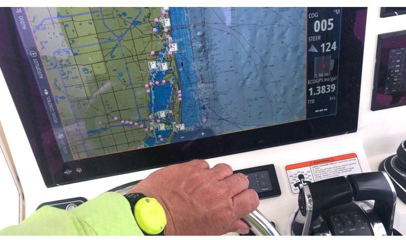
The ACR OLAS Guardian is a wireless engine kill switch and man overboard alarm system
