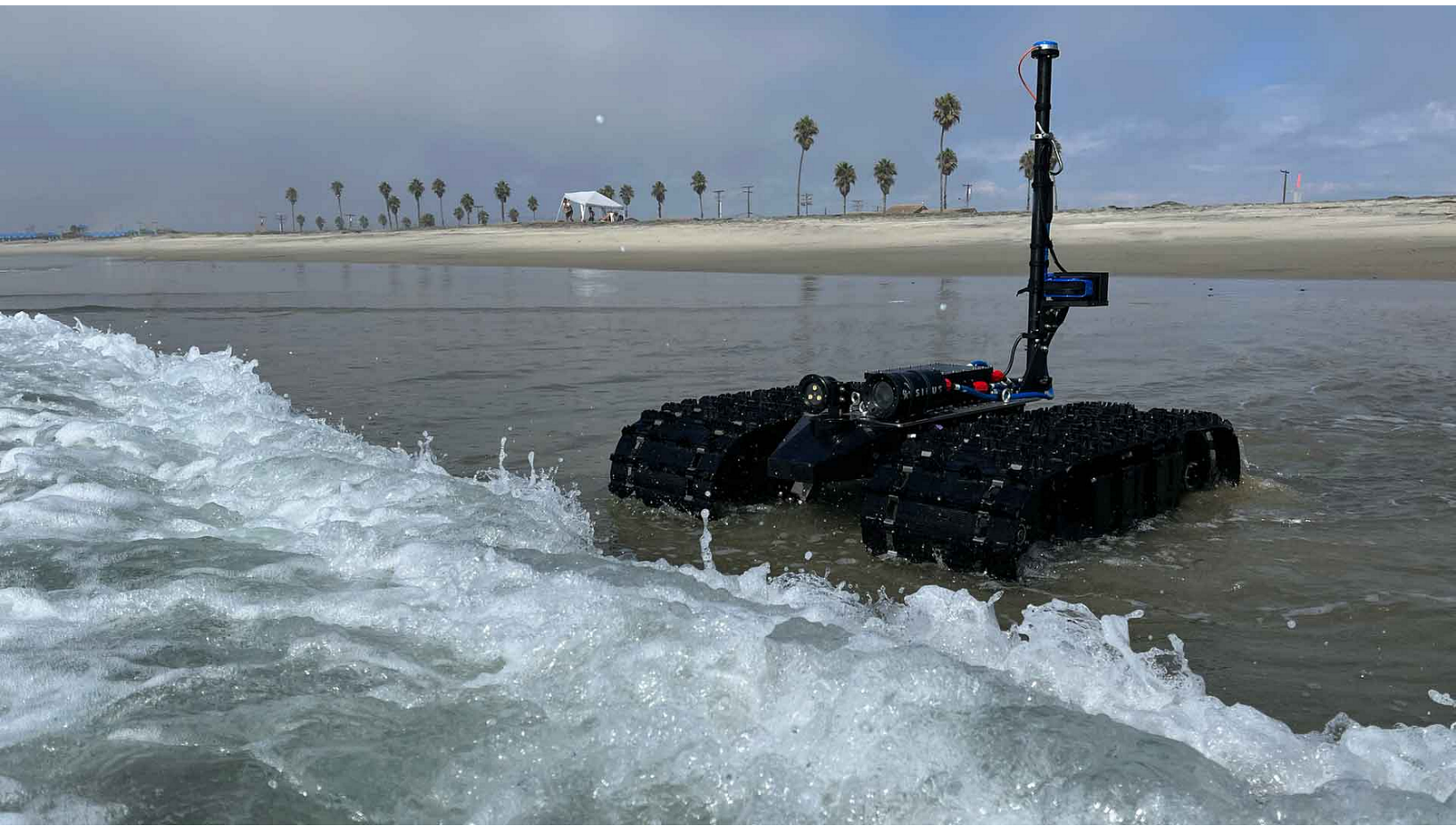
Bayonet amphibious ground vehicle transiting from the beach into the ocean
