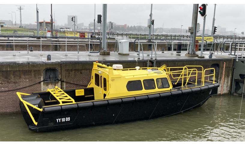
Tideman Boats' latest pilot vessel is destined for an active working life with P&O Maritime Logistics in Mozambique, equipped with an array of cutting-edge Raymarine electronics
