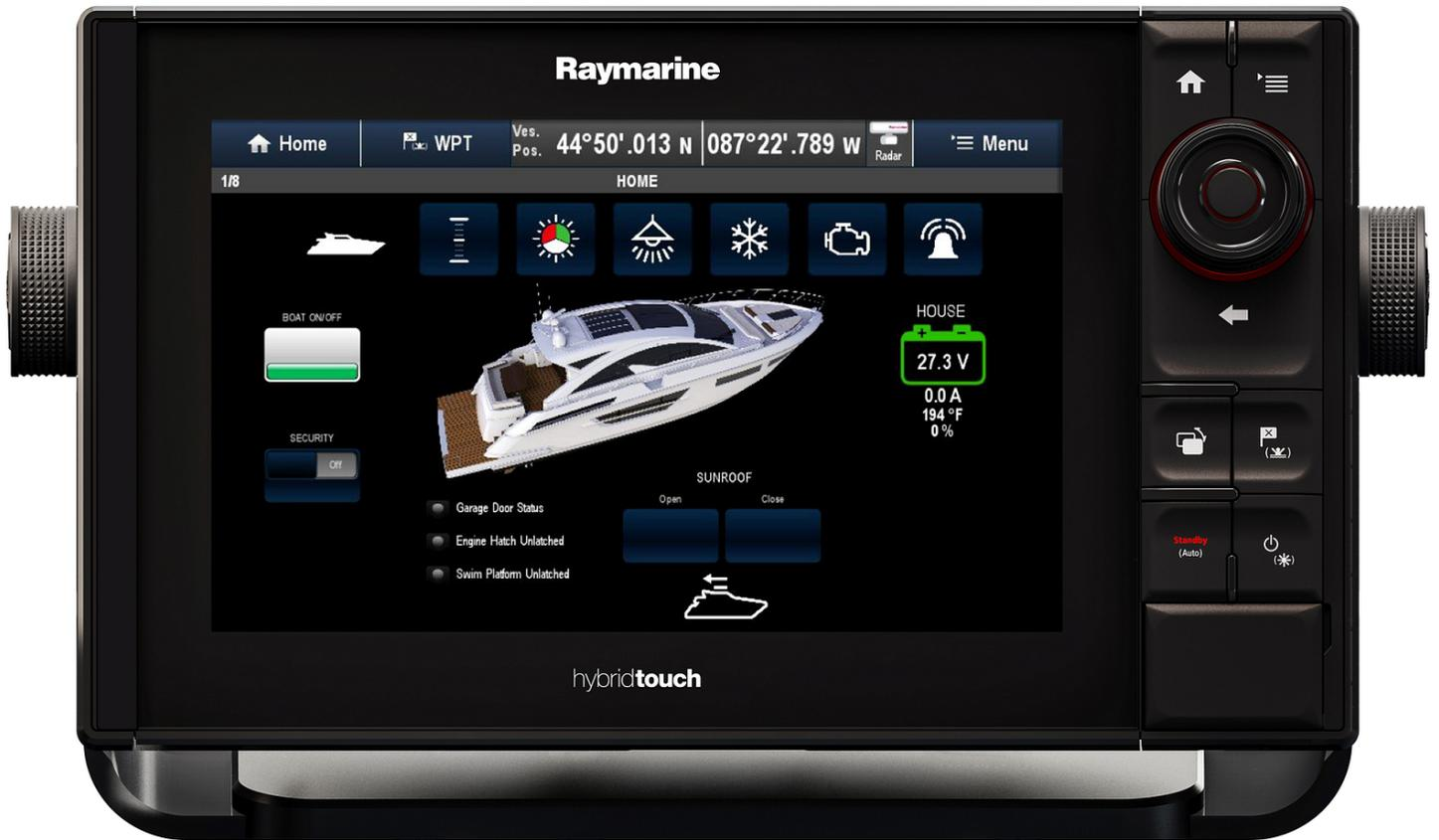
Digital switching makes it easy and intuitive to control all of the interior and exterior lighting on this high-performance centre console powerboat.
